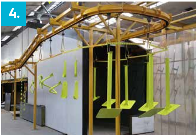
4. Painting Process – all parts are primed and powder coated in house through our paint plant.
