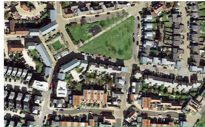
New Hall offers a network of direct permeable streets linking to key destinations and public spaces within the development.
