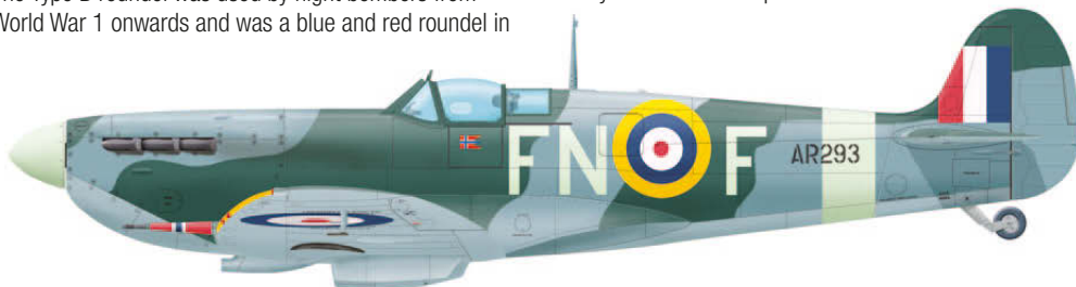
A Spitfire Vb from 331 (Norwegian) Squadron at North Weald. It has the Type A1 Roundel on the fuselage, and is finished in the 1941 Day Fighter Scheme of Dark Green and Ocean Grey top surfaces with Medium Sea Grey under surfaces, Sky squadron codes, tail band and spinner, along with yellow leading edges to the wings. The cannon housings have bands painted in the Norwegian national colours
