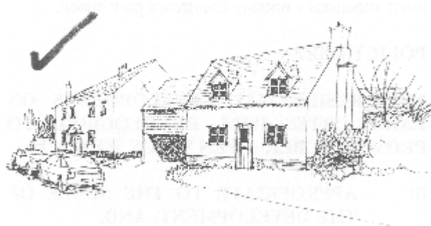
Car parking to the rear of the house enables building to be brought forward increasing enclosure of the street.
