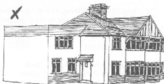
Large, flat-roofed side extensions are unacceptable
