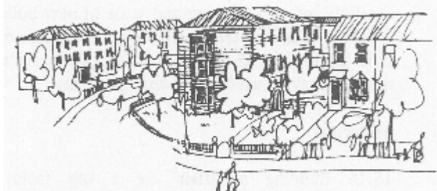
Flats redesigned to look onto all frontages with shrubs set back to allow clear vision around corner
