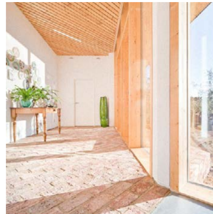
Manor Farm (Oxfordshire) by Transition by Design Extension to a listed Georgian country house that provides the home with new kitchen, dining room, garden room and utility spaces and follows sustainable design principles. The solar gains are optimised to the south allowing light and warmth to pour into the garden room yet protected in excess summer heat by the oversailing roof
