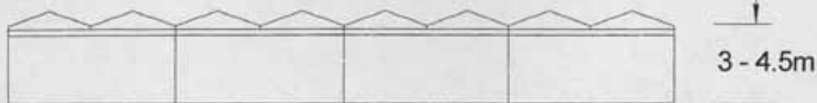
Double span Venlo type - 6.4m from post to post.
