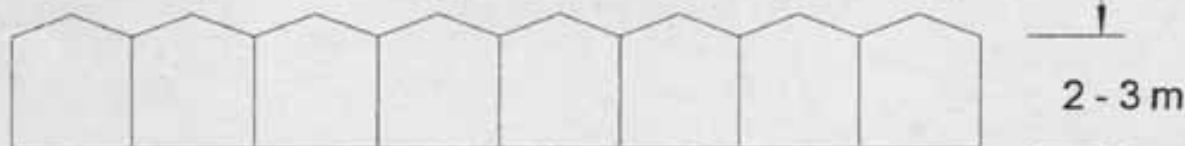
Single span Venlo type - 3.2m from post to post.
