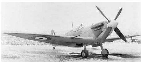
Spitfire Mark VI, AB200, was a trials aircraft at Supermarine's Eastleigh works, Southampton, after being fitted with wide span wings. Following tests at the Aeroplane and Armament Experimental Establishment at Boscombe Down, AB200 joined 124 Squadron for operations at North Weald.
