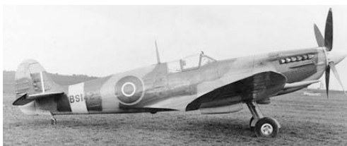
Spitfire Mark VI, BS142, at Eastleigh after modification by Cunliffe Owen, shortly before joining the High Altitude Flight (later renamed the Sub Stratosphere Flight) at Northolt. The compressor intake is visible under the exhausts. BS142 transferred to 124 Squadron at North Weald in January 1943. It subsequently also served with 331 (Norwegian) Squadron at the Airfield.
