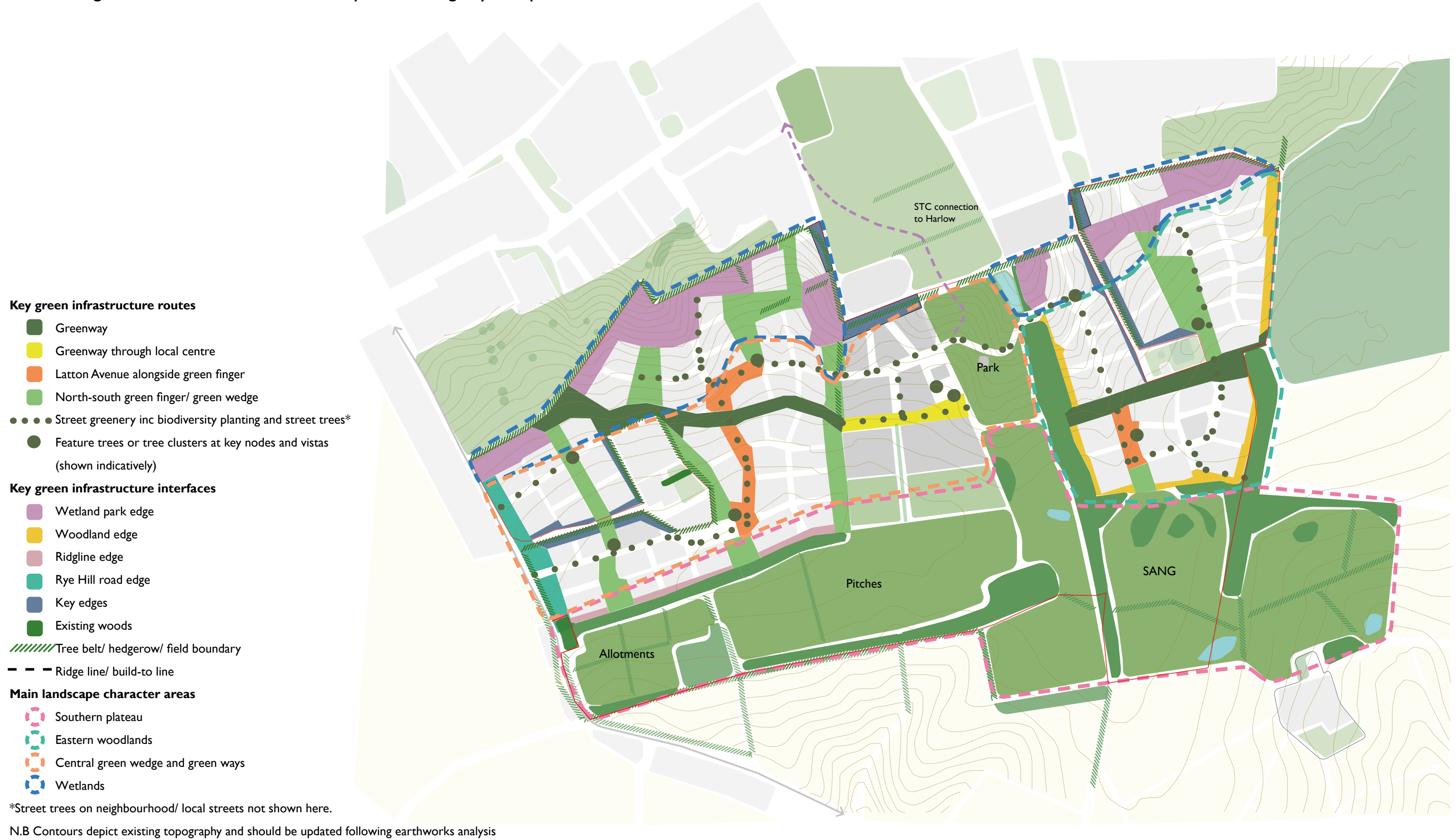
Illustrative green infrastructure framework plan showing key components, routes and character areas
